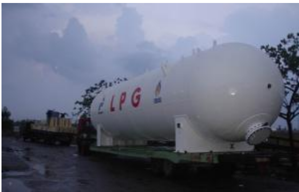
Deliver 50 Tons LPG Static Storage tank
