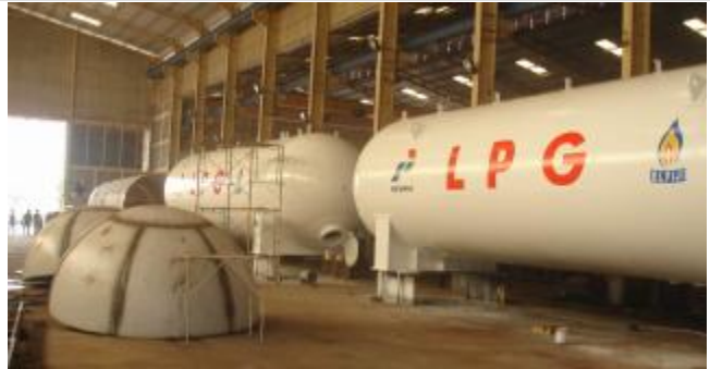
Manufacturing 50 Tons Static Storage Tank
