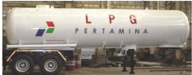
Manufacturing 15 Tons Land Transport Tank
